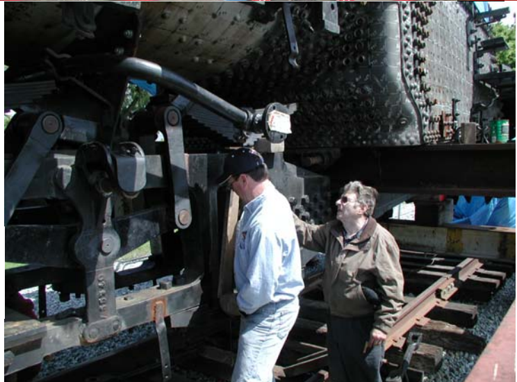
Robert Franzen and Art Randall inspecting the 2479 for future installation of the shoes and wedges.
