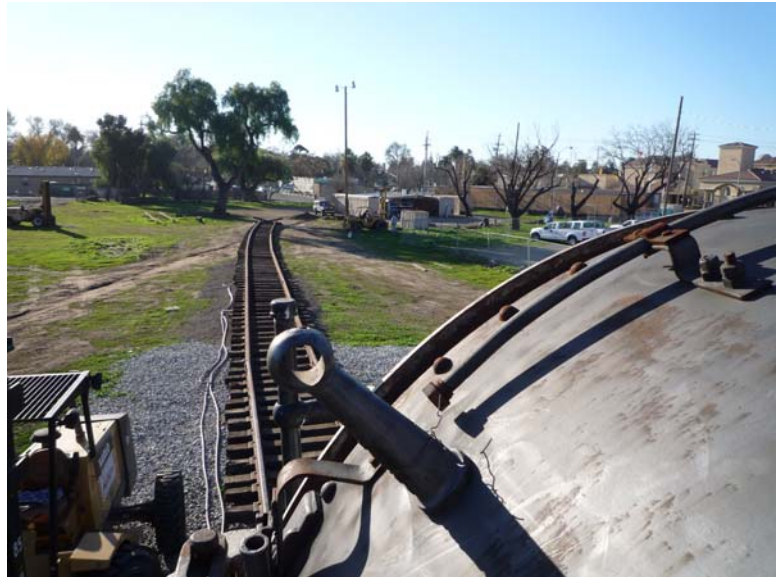
The CTRC Railroad as viewed from the 2479. The hose you see on the ground supply compressed air to the leading truck to brake the locomotive.
