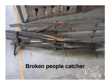
The people catcher inadvertently dropped on 3/26 and snagged an obstacle. Many of the iron parts were bent. Because this has happened a number of times, we're seeking help through ARM to make it more reliable when we repair it.
