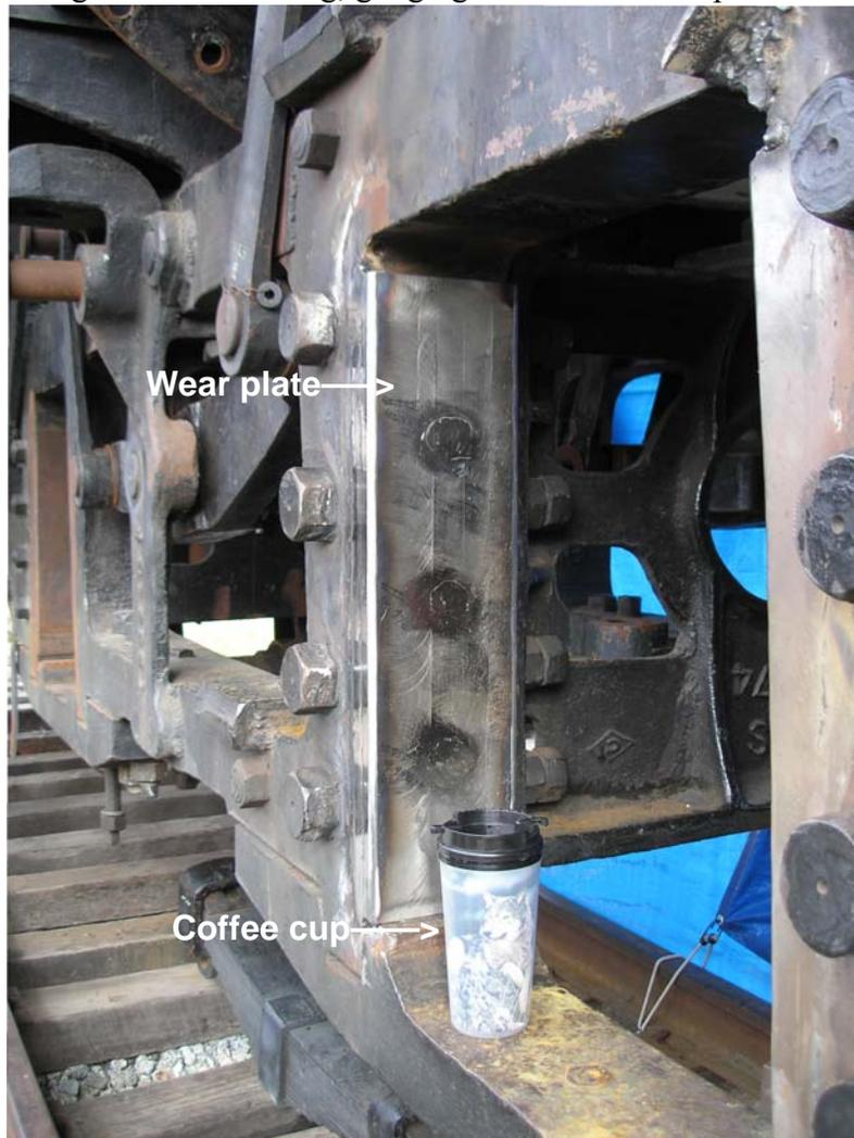
chining a new wear plate, test fitting and finally weld the new wear plate into place. In addition to the wear plate a number of defects were correct in the frame and the other wear plates as well. This process turned out to be very labor intensive. Additional the spring hangers are being machined to height.
