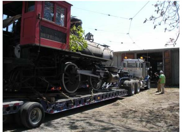
**Using** Taylor's truck for braking, Buttercup was rolled off the trailer. For the final positioning in the trolley barn, a special extended reaching forklift from A-Tool Shed was utilized. The special ramp constructed by John Blaine performed flawlessly as the height clearance at the barn door was near zero!
