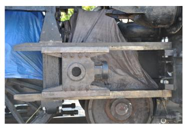
Back in May, 2010, the position of the right crosshead guides to the center of its piston rod were measured and found to be significantly out of line at the end of stroke. When the upper and
