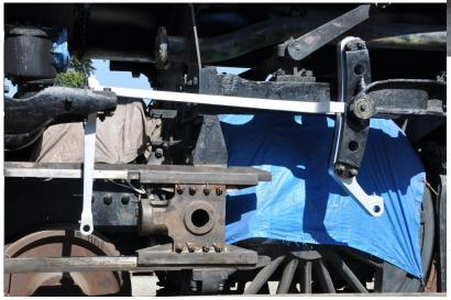
Left side repairs and assembly were not as complicated. The left crosshead required weld up of the combination lever pin holes as they were well oversize. These holes were then machined and new bushings fabricated. Since the lower bronze surface of the crosshead did not require any work, setting the height of the crosshead to the piston rod was straight forward. Assembly of the reverse link, combination lever and radius rod presented none of the problems experienced on the right side.
