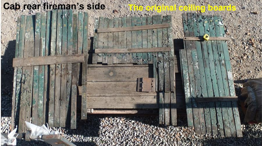
the lumber to the required thickness. It was quickly learned that the proper tools were not available and a wood shop was contracted for this work. Returned material was just slightly over the needed three-quarter inch thickness. Jerry Lane allowed the use of his planer to mill the planks down to the three-quarter inch thickness. Planks are now being sanded and prepared for the next step, milling tongue and groove edges.
