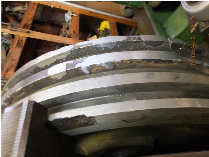
An additional layer of weld was applied to the second of four thin areas on the fireman's side of the firebox's roof sheet. Grinding of the welded area has begun. Ultra sound thickness measurements were taken in some areas. Results look good but more grinding is required.
