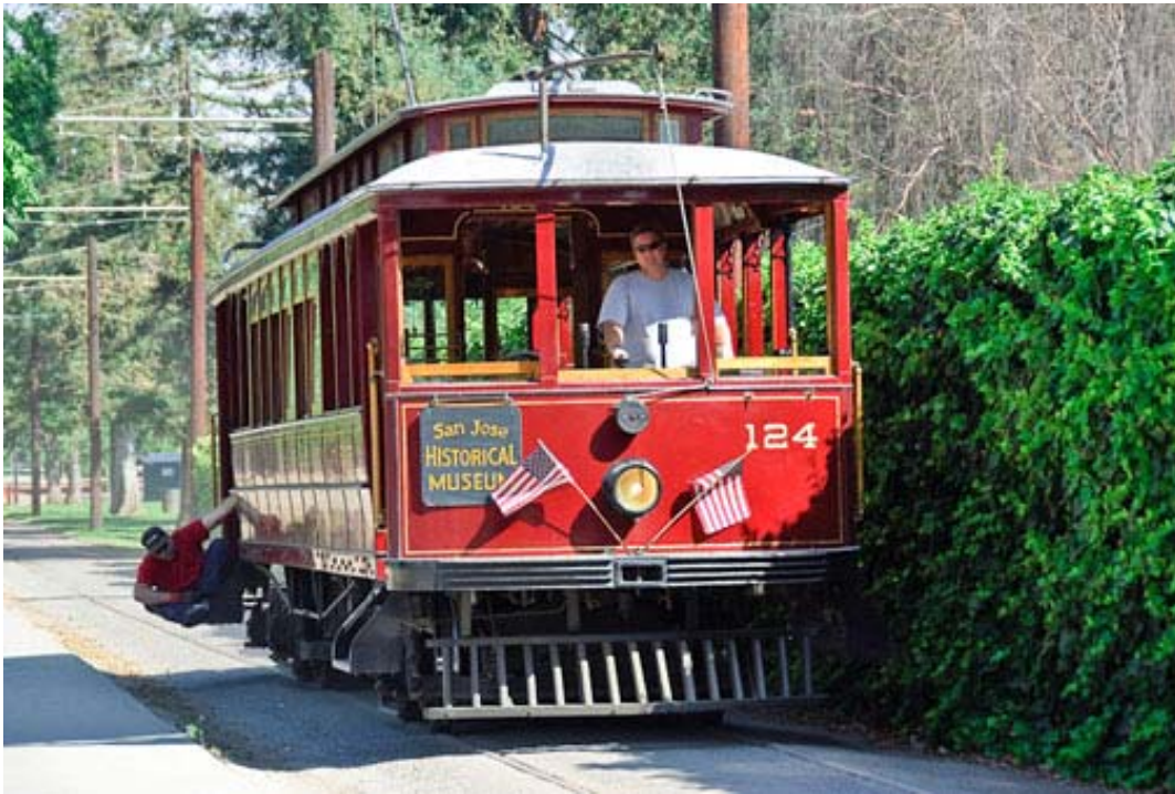
Steve watching for excessive wheel-to-rail arcing during run-in
