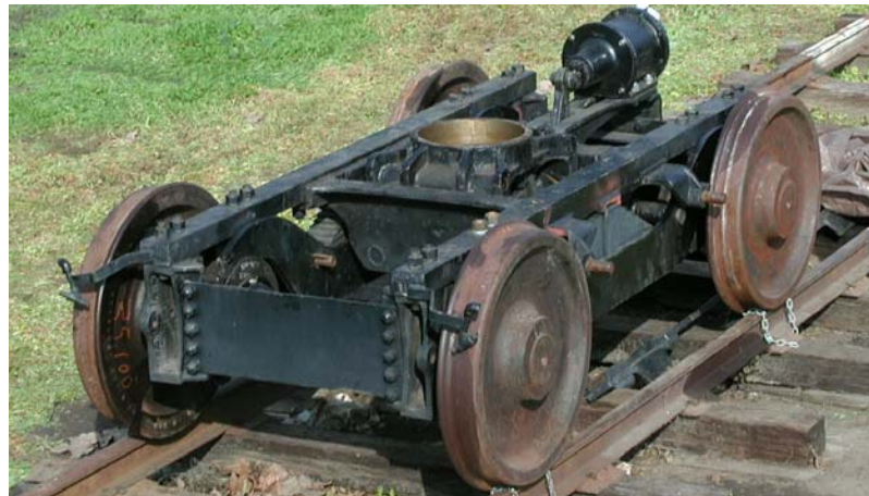
Leading truck reassembled on 17 JAN 2004 Awaiting brake rigging
